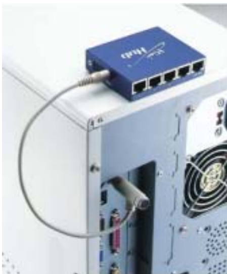
+5Vdc Power from Shared PS/2 Keyboard
